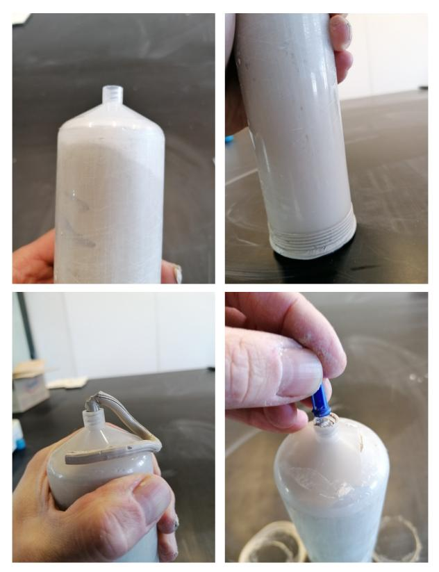
Push in the piston. Remove excess material and attach the nozzle.
