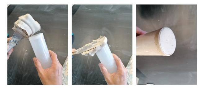
Use the putty shovel to fill the tube. Try to keep air bubbles from being trapped in the material. Leave some space for the rubber piston.
