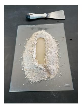
Put the clay powder on the glass plate. Create a pit for water. Pour the water into the pit and wait for 5 minutes. Use the putty shovel for mixing. Mix until all material is completely uniform. The result should be slightly sticky but not runny.
