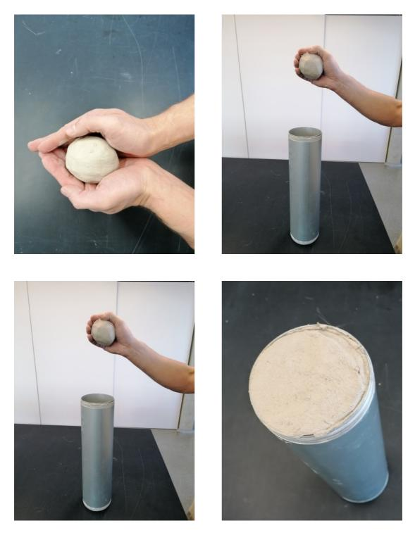
Close both ends of the container. Since the tube has symmetrical ends, you can use it both ways. Just be sure that the cap for pressing air goes behind the piston and the clay exiting cap is against the material.
